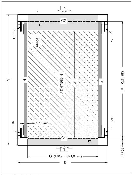
Figure 2: Mechanical requirements
